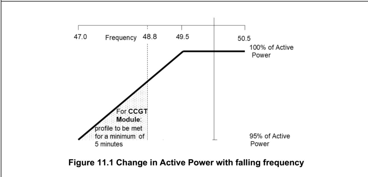
**Figure 11.1 Change in Active Power with falling frequency**
