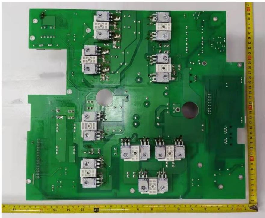
Filter Board – Component Side
